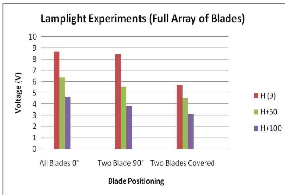
When the full array of blades were all placed at a horizontal angle and tested at a distance of 9cm from the light source, the maximum voltage
