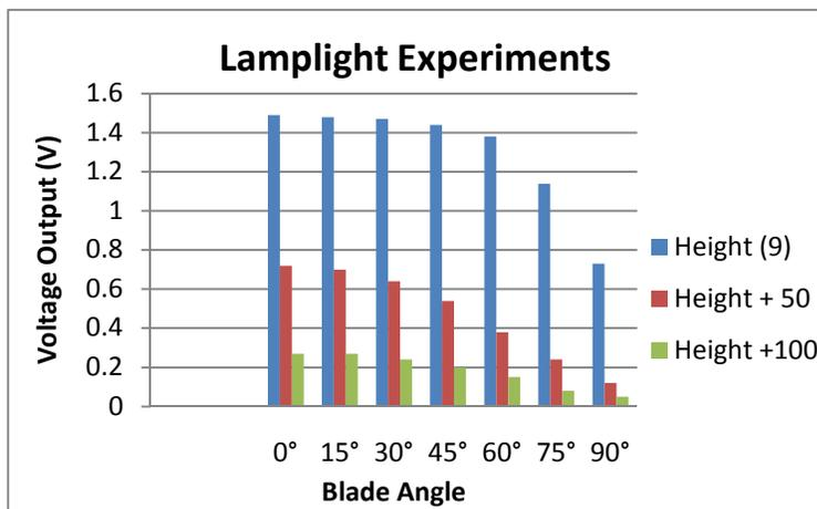
In testing a single blade at different angles and with different light intensities, the voltage reading decreased quickly, indicating that the degree of incidence, which is the angle at which the light hits the solar
