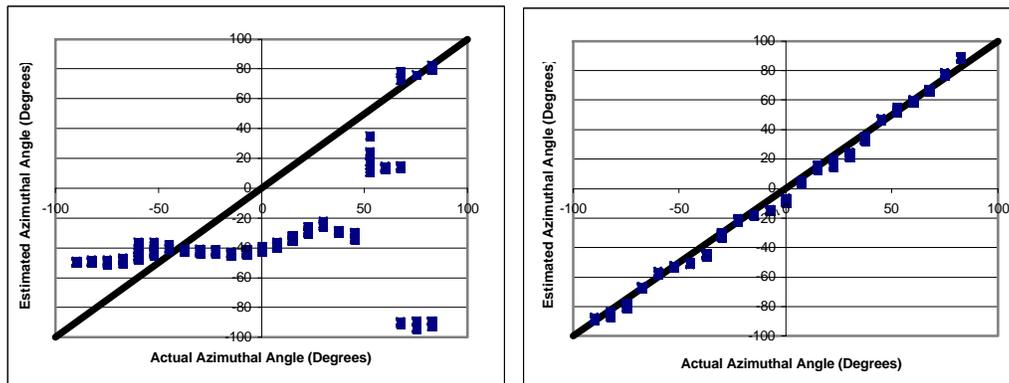
The system was very susceptible to environmental noise. Use of multiple samples compensated for some of the noise, but this did not eliminate biases introduced by such acoustical effects as reflected signals from fixed surfaces in the vicinity of the array.
