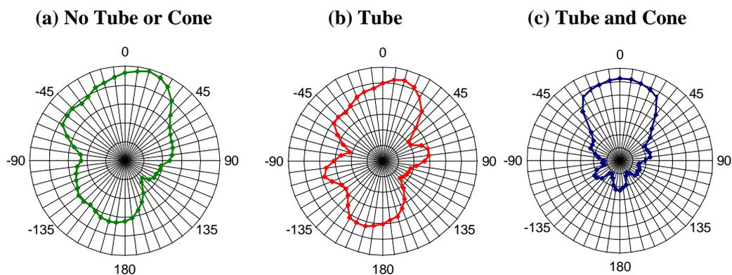
The plot shown in figure 1c was obtained using the design I selected for the static array. The housing had a 2 cm wide tube that was 4 cm long, and a 7 cm long funnel that was 10.5 cm wide. Between  $-52.5$  degrees and  $+52.5$  degrees the signal amplitude is a smooth curve that resembles a parabola. Therefore, a quadratic function can be used to model the data, and its maximum value will be near 0 degrees.
